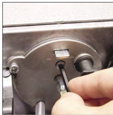
fig. 15 : Combustion head adjuster screw
