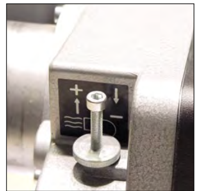
fig. 16 : Air flow adjuster screw (fine tuning)
