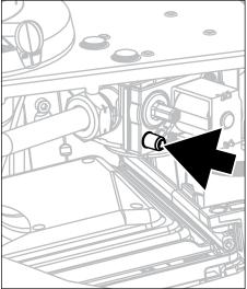
Adjustment screw CO<sub>2</sub> Figure 15.1.b
