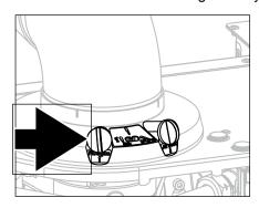
Measuring point CO<sub>2</sub> Figure 15.1.a
