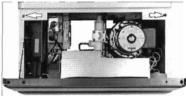
To remove the side panels which make up the case, loosen the lower screws "A" and proceed in the same way as for the front panel.
