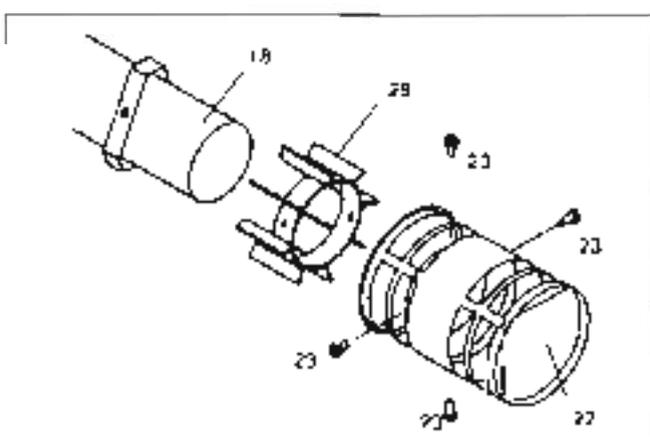
insert the exhaust pipe into the suction pipe so that the wind-resistant flue vent contacts the rim which is located on the inside of the suction pipe:
