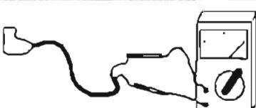
ref. 5 To check the continuity of a cable, disconnect the cable from its circuit and measure the resistance when the two ends of the cable are connected. The resistance should be zero ohms with the tester set to the ohms function
