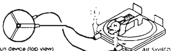
ref. 13 The tubes between venturi device and air switch must be connected as shown
