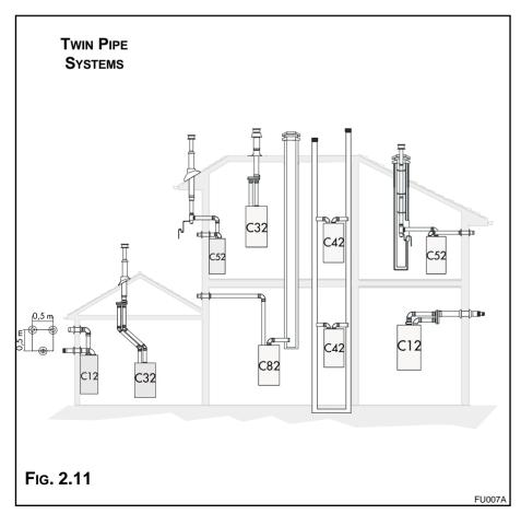
In calculating the lengths of the pipes, the maximum length "L" must also take into consideration the values for the exhaust/air intake end terminals, as well as 90° elbows for coaxial systems.
