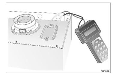
In the boiler, it is possible to monitor the correct operation of the flue exhaust/air intake, checking for a loss of general pressure in the system. Through the use of a differential manometer connected to the test points of the combustion chamber, it is possible to detect the  $\Delta P$  of operation of the air pressure switch.
