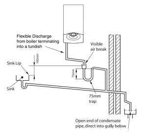
3. External termination of condensate drainage pipe via internal discharge branch (e.g. sink waste - proprietary fitting).
