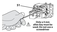
Set the content by turning the screw about a 1/4 of a turn then wait after each change for approximately 1 minute for the CO2 value to stabilise, then repeat.
