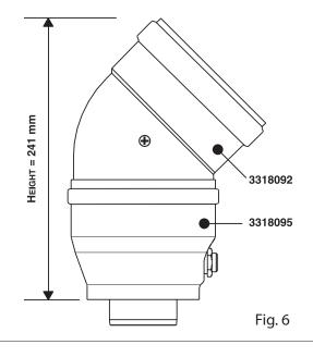
Once the boiler has been positioned on the wall, it is necessary to insert the Ø80/125 adaptor (Fig. 5) for both horizontal and vertical flue runs into the boiler flue socket (not supplied with flue kit - Part No 3318095).
