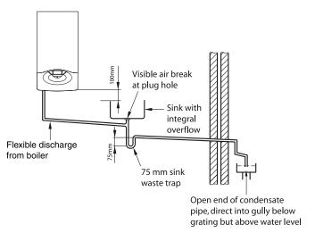
4. External termination of condensate drainage pipe via condensate siphon
