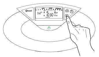
If the  ${\sf I}{\sf NFO}$  button is pressed, a menu is accessed which enables the data listed in the table below to be displayed.
