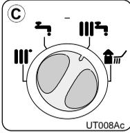
The boiler is fitted with a selector knob "C" which allows you to switch between winter < III' 2' > and summer < 2' > and also heating only < III' > operating modes and vice versa. When the knob is set to < III' 2' >, the boiler can serve the dual purpose of providing heat and/or hot water for domestic use.
