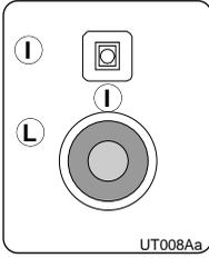
To turn off the main burner, simply press the On/Off switch “L”; the green L.E.D. “I” will also turn off.
