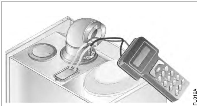
The discharge/ventilation of the exhaust fumes can be monitored to check for losses in general pressure in the system. This is done to eliminate the cause of lighting failure with the main burner not indicated by a shutdown status.
