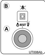
does not light within the pre-set safety time limit, the red "B" L.E.D. will light up. To reset the ignition system, the reset button "A" must be pressed. Should the system fail to light a second time, check to make sure that the gas cock is open. If the problem persists, contact one of our Authorised Service Centres for assistance.
