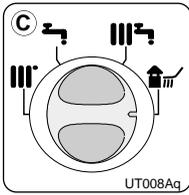
The “C” Summer/Winter/Flue Test selector knob can be set to < III > to bypass temperature adjustment on the heating circuit for the purpose of analysing the fumes produced by combustion.
