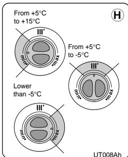
**ADJUSTING THE HEATING TEMPERATURE**
