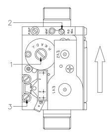
The CO<sub>2</sub> % is reduced if the screw is turned anti-clockwise and increased when it is turned clockwise.
