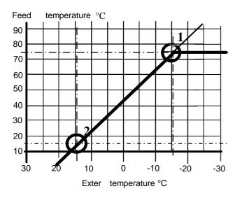
**STEP 2.** Now the associated external temperature, by which this max. supply temperature is required, needs to be programmed in.
