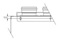
For maintenance and service purposes the front and underside of the appliance need to be accessible; both sides need to be at least 20mm from a wall or cupboard wall.
