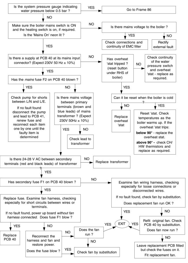
*Foot Note:* Presence of live supply on a terminal may be checked with a multimeter set to the appropriate AC range (apply the other probe of the meter to mains neutral, e.g. on terminal N of the programmer terminal strip).
