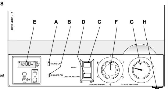
Check that the overheat thermostat has not tripped - press button (H) to reset.
