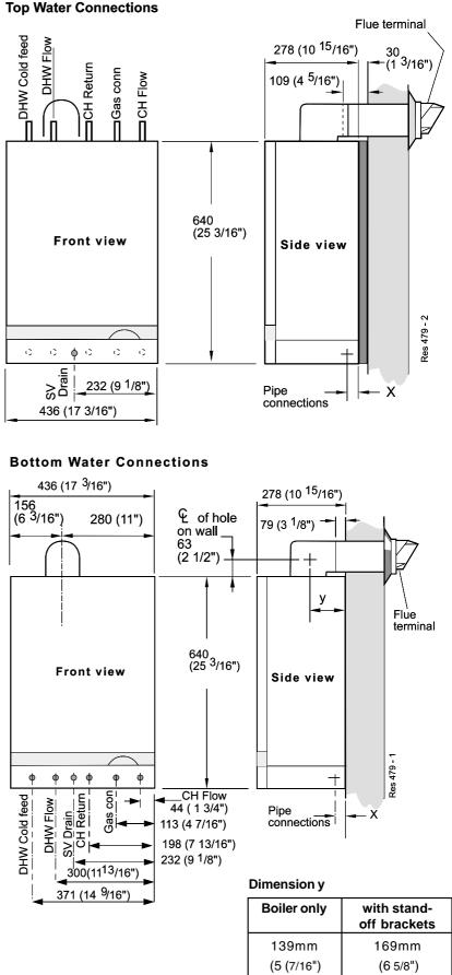
Distance X is 20mm for DHW pipes and safety valve outlet. Distance X is 23.5mm for CH pipes and gas inlet.
