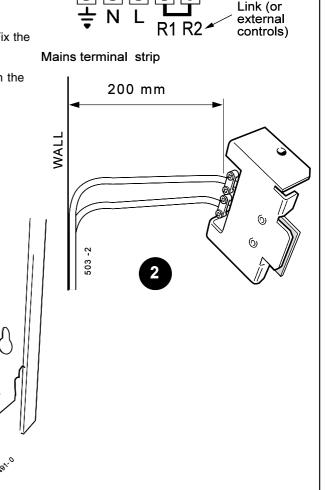
**Note.** Ensure that the lengths of the current conductors are shorter than the earth conductor so that if the cable slips in its anchorage the current carrying conductors become taut before the earth conductor.
