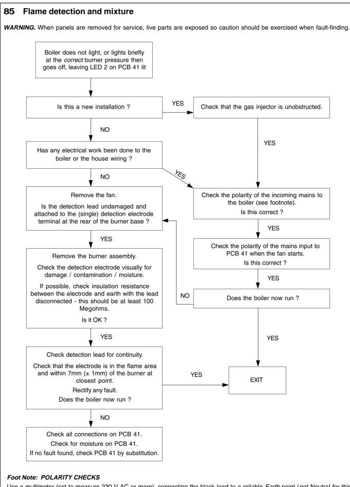
Use a multimeter (set to measure 230 V AC or more), connecting the black lead to a reliable *Earth* point (*not Neutral for this particular test*).
