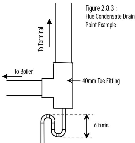
Figure 2.8.3 : Flue Condensate Drain Point Example
