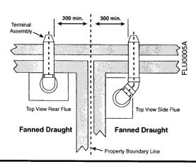
Terminal Position with Minimum Distance (mm)
