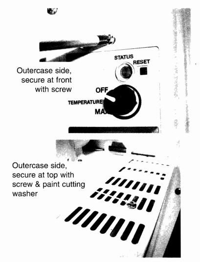
**Important:** The screw and paint cutting washer are used to earth the outercase side.
