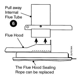
4.8 Flue Hood & Internal Flue Tube
