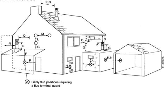
Where a horizontal flue is sited less than 2m above a balcony, above ground, or above a flat roof to which people have access, a suitable terminal guard must be fitted. This serves two purposes, to protect the terminal against damage or interference and to protect passers-by. A terminal guard is available (Sales Code: PTERMGUARDEF), this should be fitted centrally about the terminal.
