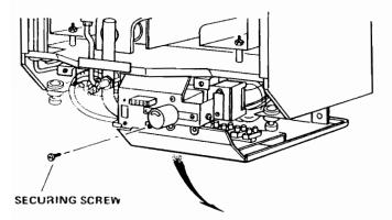
FIG. 22 ACCESS TO THE BOILER ELECTRICAL TERMINAL BLOCK The boiler terminal block which is situated in the control box is not designed to accept wiring from all the on site controls and therefore the installer will usually need to incorporate a suitable junction box. This may not be required if a Potterton Electronic Programmer is used as this incorporates a junction box. The principle of wiring is shown in FIG. 21.
