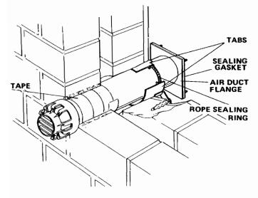
Engage four screws from accessory pack 'C' into the pre-drilled holes in the terminal and screw fully home.
