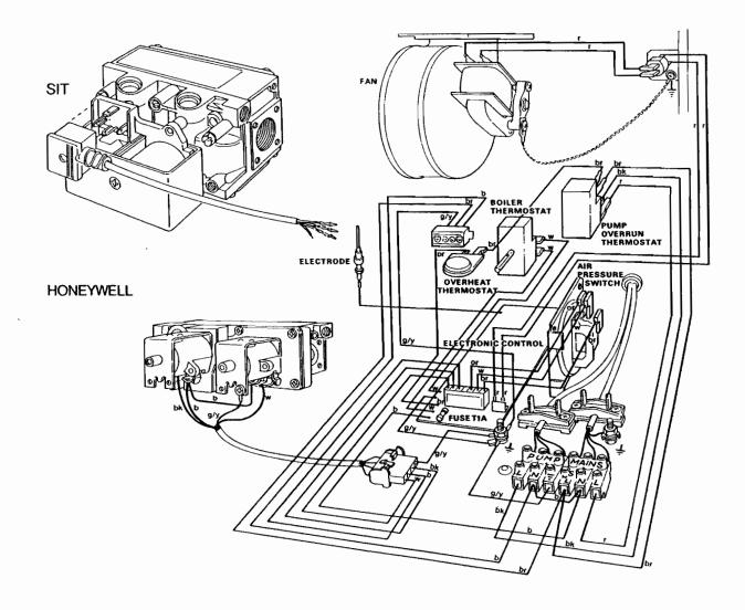
FIG. 27 BOILER WIRING DIAGRAM.
