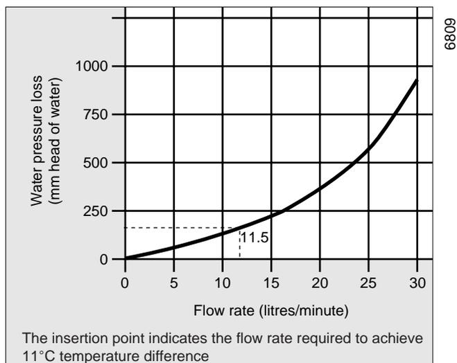
The insertion point indicates the flow rate required to achieve 11°C temperature difference
