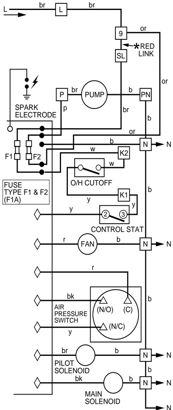
\* Remove red link between 9 and SL when fitting a time control etc (if no switch is fitted, link will make the circulation pump run constantly)
